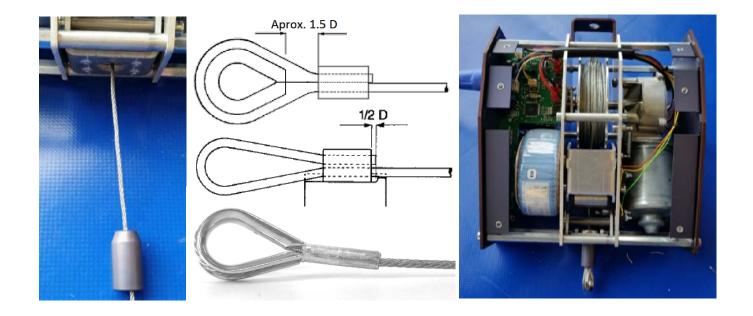
24. Mount the middle plate on the winch again and fasten it with the six 3mm hexagonal socket screws per plate. Tighten them slightly
