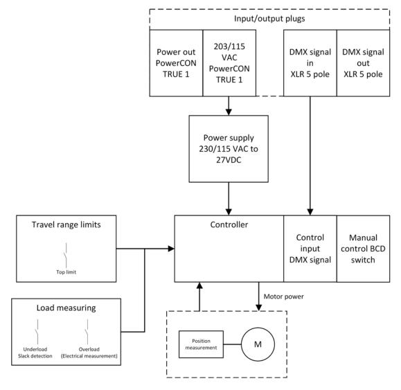
Block diagram of the control system of the winch.
