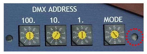
The position is set on the DMX channel 1 and 2, which controls the rough-and fine-position. Where 100 % is the soft TOP limit and 0 % is the soft BOTTOM limit.
